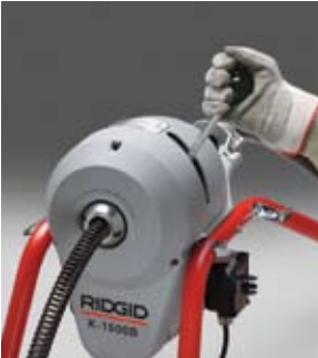
Engage clutch, cable spins.
