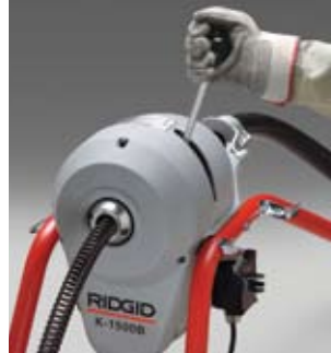
Release handle, cable stops instantly.
